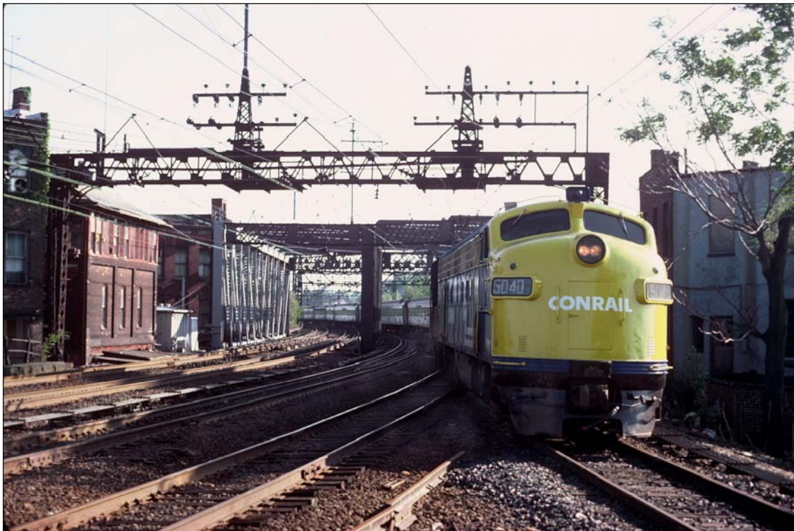
Former New Haven Railroad FL-9 Locomotive Renumbered #5040 in Conrail Dress Leading a Northbound Danbury Train Past Berk Tower in 1978 Tower Operator is Standing in Shadow "Hooping Up" Clearance Card with any Train Orders Mechanical Pipe Line is Visible between Mainline Tracks 1 and 2, and to Right of Locomotive Photo by J. W. Swanberg
